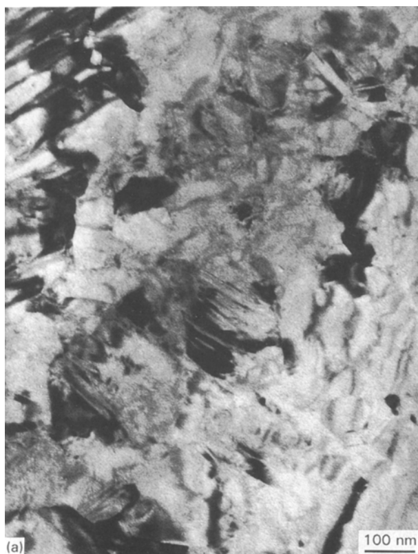
Figure 4 TEM pictures of ED Ni foils having thicknesses of about 4 to 5 \mu\text{m} and prepared with (a) i_{\text{dep}} = 100 \text{ mA cm}^{-2} (a different area of the same sample to that in Fig. 2a) and (b) i_{\text{dep}} = 500 \text{ mA cm}^{-2} .
