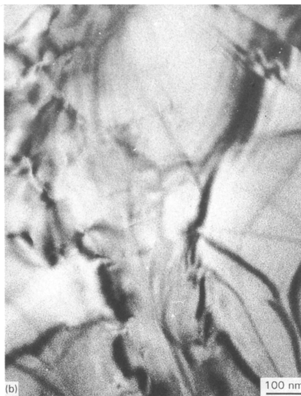
Figure 4 TEM pictures of ED Ni foils having thicknesses of about 4 to 5 \mu\text{m} and prepared with (a) i_{\text{dep}} = 100 \text{ mA cm}^{-2} (a different area of the same sample to that in Fig. 2a) and (b) i_{\text{dep}} = 500 \text{ mA cm}^{-2} .
